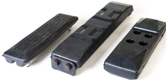
NTP rubber pads are available in three different versions; Chain-on which is replacing the steel shoe and bolted directly on the chain, Clip-on is attached with clips to the existing shoe, and Bolt-on which is bolted through pre-drilled holes in the shoe.
